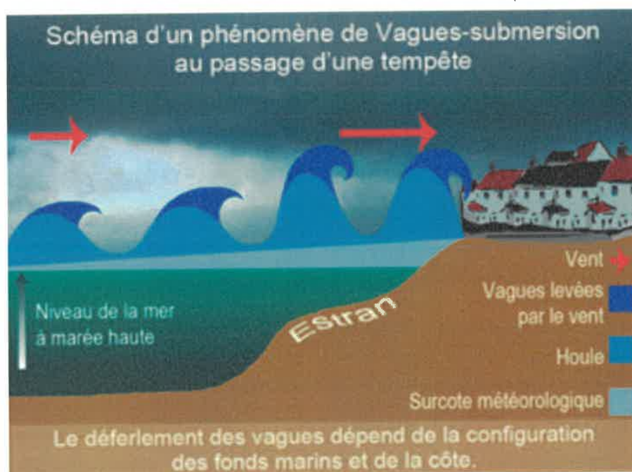
Figure 17: Schéma de submersion marine
